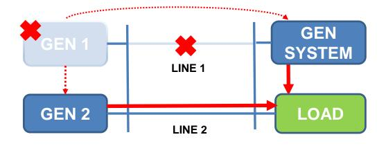
**GEN 1** is part of remedial action scheme and trips off if **LINE 1** or **LINE 2** go out
