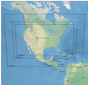
Figure: WRF simulation domains. (from “Overview and Meteorological Validation of the Wind Integration National Dataset Toolkit”)
