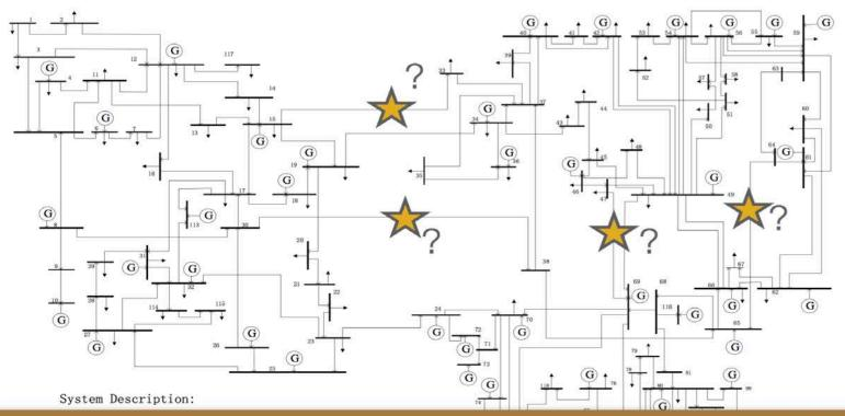
Make a decision about how to operate now while considering all N-1 possibilities for transmission element failure.
