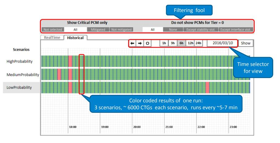
Color coding: Acceptable; Near critical; Critical; Voltage collapse which could be mitigated by load shedding
