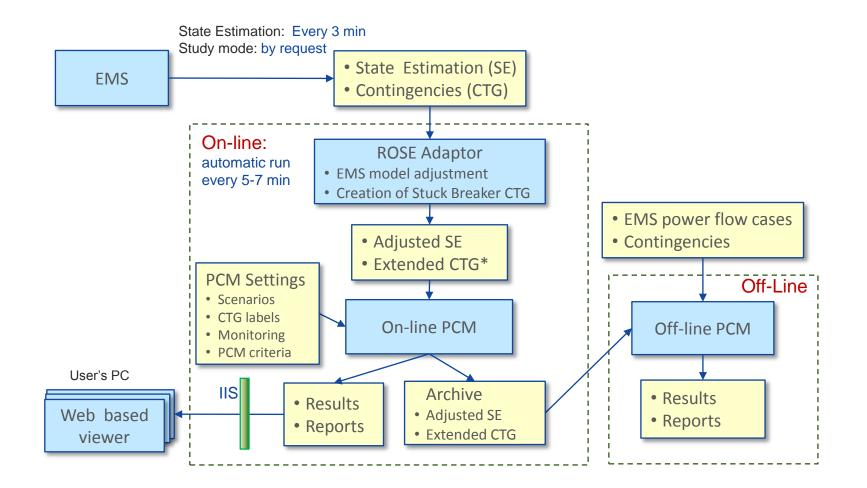
\* Extended CTG include selected N-2 used in Day-Ahead processes and all Stuck Breaker. Total ~6,000 x 3 = 18,000 CTGs
