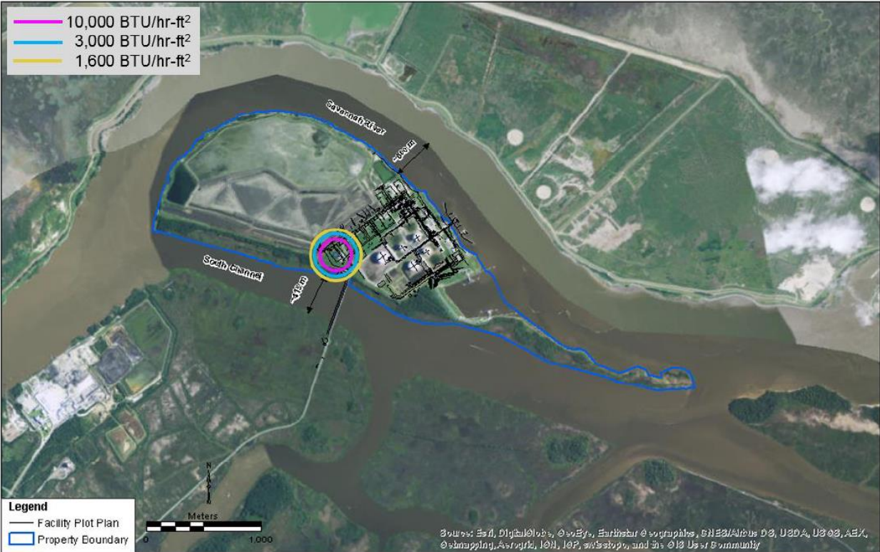
Figure 2.8.6-10 – Thermal Heat Fluxes for a Jet Fire from a Mixed Refrigerant Release
