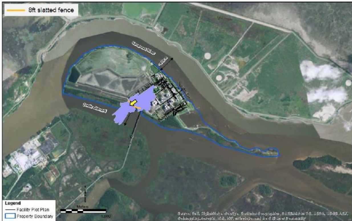
Figure 2.8.6-5 – Jetting and Flashing Scenario from the LNG Rundown Line at Liquefaction Unit Closest to the Property Line Adjacent to the South Channel with Vapor Fencing (1 m/s)
