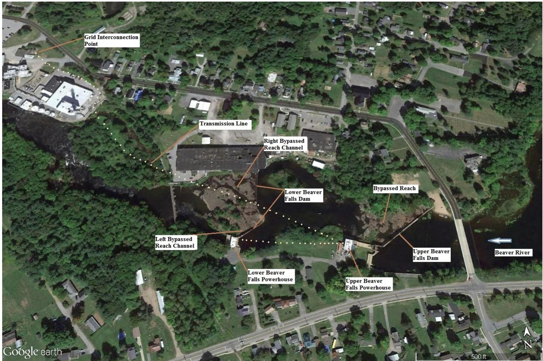
Figure 2. Project location and facilities of the existing Upper and Lower Beaver Falls projects (Source: Google Earth 2018, as modified by staff).
