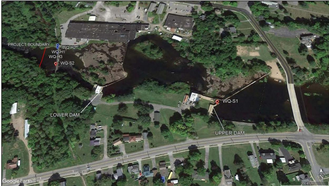
Figure 5. Continuous water quality monitoring stations at the Beaver Falls Project (Source: license application, as modified by staff).
