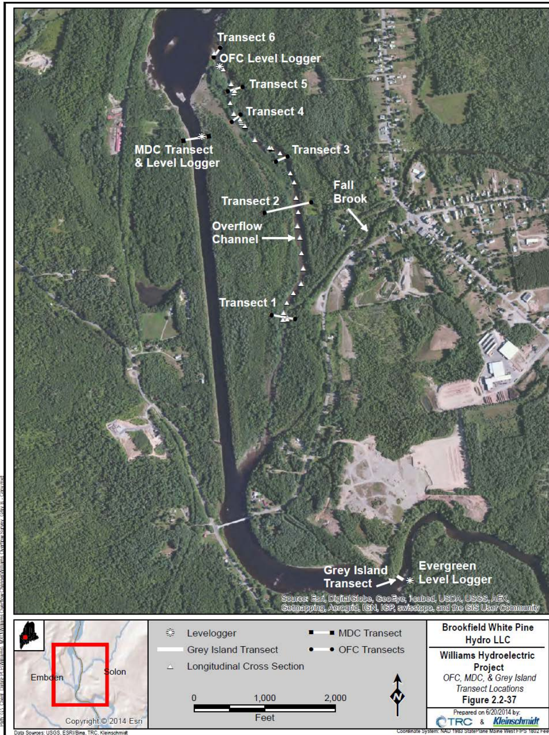
Figure 11. Kennebec River and overflow channel downstream of the Williams Project. The figure shows the transect and centerline streambed elevation (i.e., “longitudinal cross section”) measurement locations that White Pine Hydro studied in the overflow channel (Source: ISR Figure 2.2-37, filed June 23, 2014).
