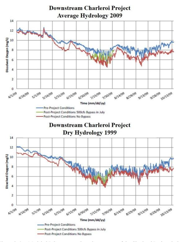
Figure 3-6. Modeled DO concentrations downstream of the Charleroi Project during an average year (2009) and dry year (1999) (Source: CDM Smith, 2015).
