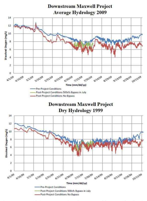
Figure 3-5. Modeled DO concentrations downstream of the Maxwell Project during an average year (2009) and dry year (1999) (Source: CDM Smith, 2015).
