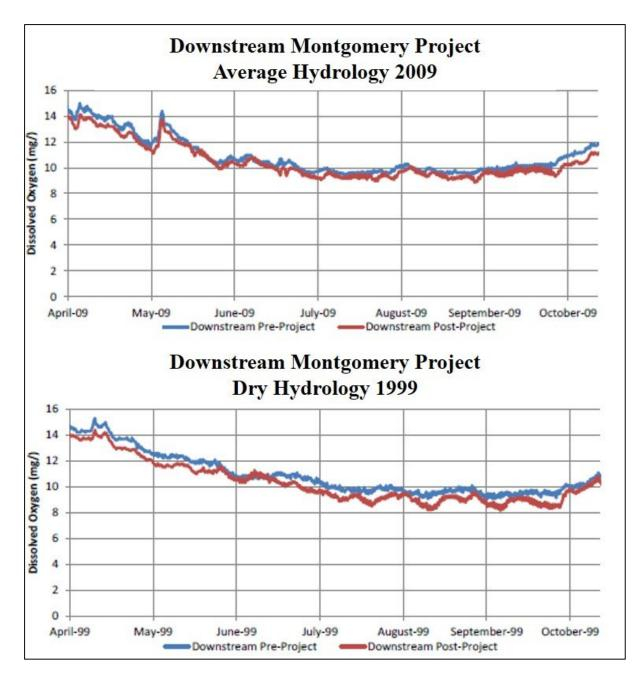
Figure 3-10. Modeled DO concentrations downstream of the Montgomery Project during an average year (2009) and dry year (1999) (Source: CDM Smith, 2014b).
