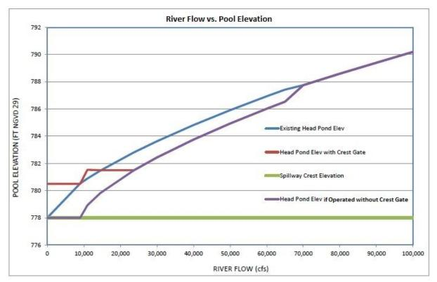
Figure 2-1. Grays Landing Project headwater rating curve for normal operation (Source: FFP Missouri 13, 2014).
