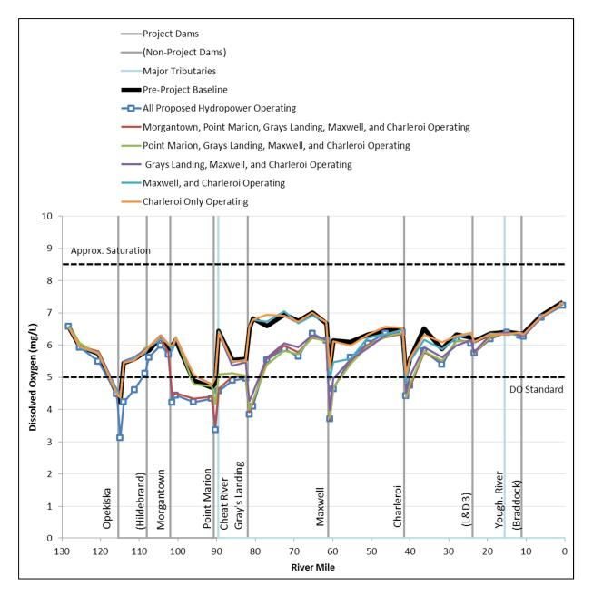
Figure 3-8. Modeled minimum DO concentrations along the Monongahela River between June 15 to September 30, 1999 (dry year) (Source: Rye Development, 2014).
