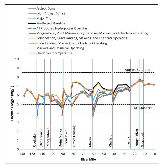
Figure 3-7. Modeled minimum DO concentrations along the Monongahela River between June 15 to September 30, 2009 (average year) (Source: Rye Development, 2014).
