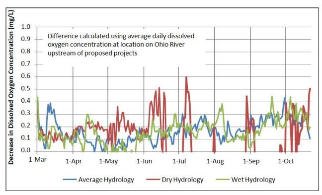
Figure 3-9. Difference in DO concentrations upstream of the Ohio River Projects, with and without the Monongahela and Allegheny River Projects (Source: CDM Smith, 2014b).
