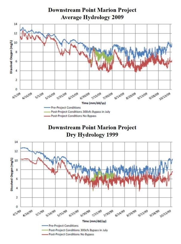
Figure 3-3. Modeled DO concentrations downstream of the Point Marion Project during an average year (2009) and dry year (1999) (Source: CDM Smith, 2015).
