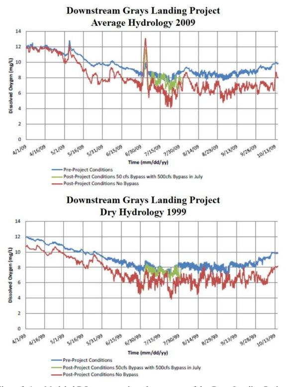
Figure 3-4. Modeled DO concentrations downstream of the Grays Landing Project during an average year (2009) and dry year (1999) (Source: CDM Smith, 2015).
