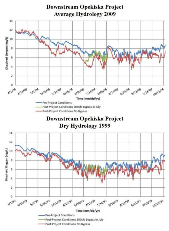
Figure 3-1. Modeled DO concentrations downstream of the Opekiska Project during an average year (2009) and dry year (1999) (Source: CDM Smith, 2015).
