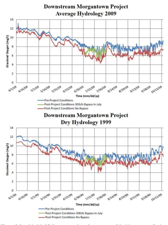
Figure 3-2. Modeled DO concentrations downstream of the Morgantown Project during an average year (2009) and dry year (1999) (Source: CDM Smith, 2015).
