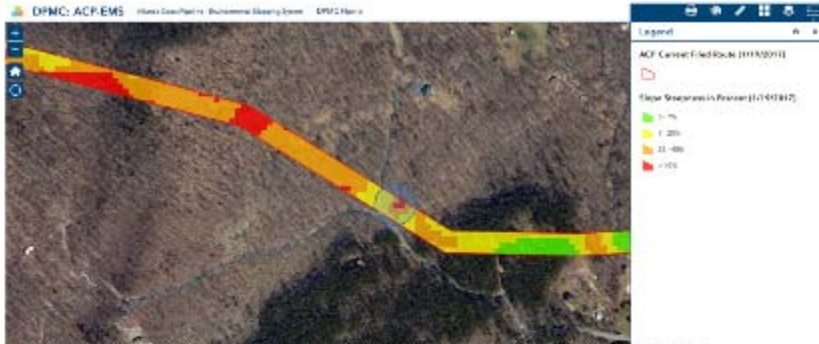
Figure 2 – Slope Steepness along proposed ACP route with blue circle highlighting the area adjacent to the western tip of the wetland within the Spruce Creek Tributary Conservation Site.
