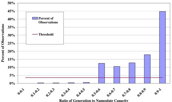
Figure 3: Histogram of Steam Turbines with an Estimated Eco-Min Ratio from 0.5 to 0.6
