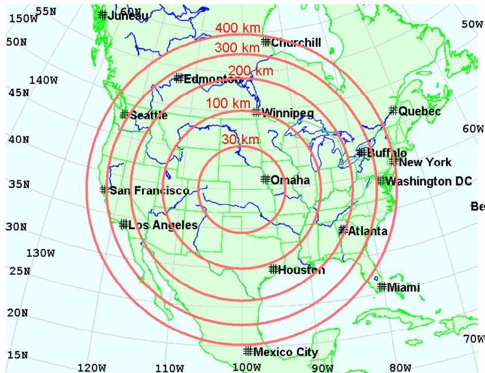
Figure 2-3. E1 HEMP exposed regions for several burst heights (red values), for a nuclear burst over the central U.S.
