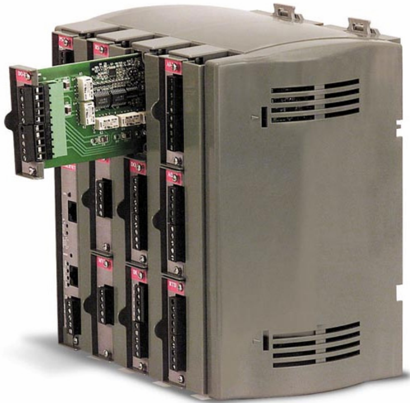
Figure 5-7. The Fisher ROC809 Remote Operations Controller. This is a PLC, such as might be used for remote controlling of a pipeline. It has a computer, and then may be configured with various I/O units: analog, binary, and communications.
