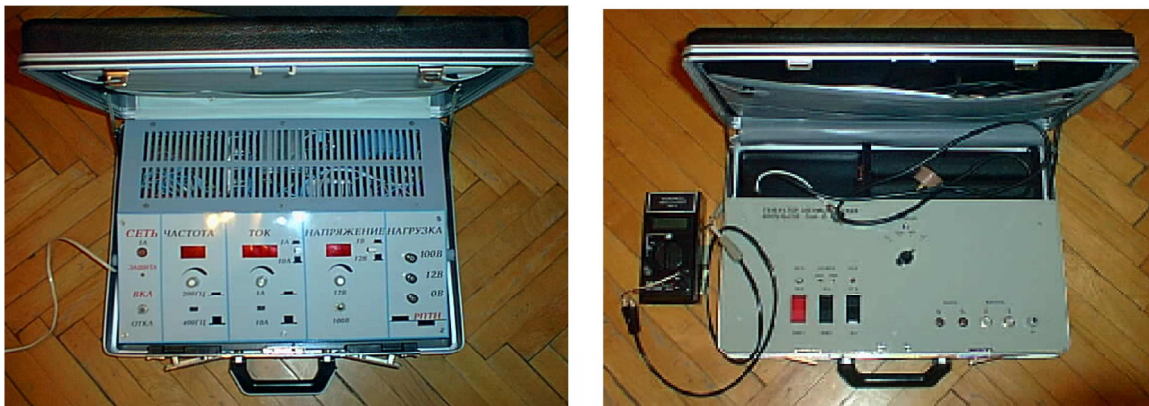
Figure 2-11. Examples of briefcase generators for producing conducted environments: CW generator (left) and impulse generator (right) [15]
