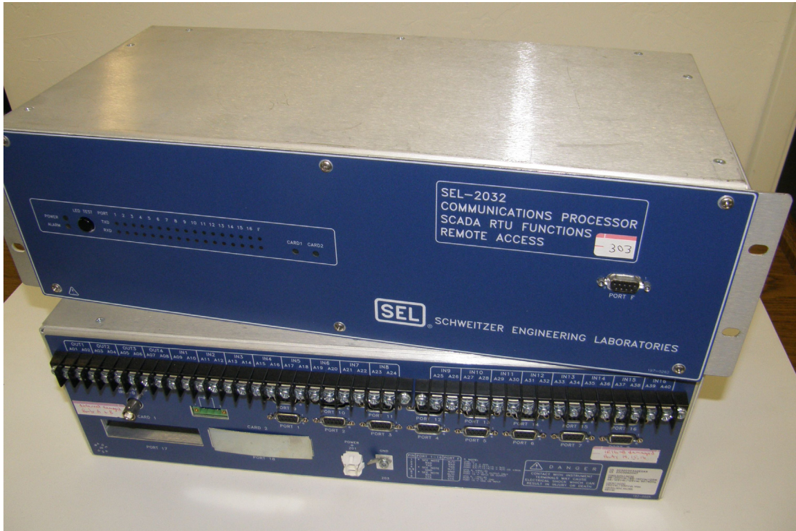
Figure 5-5. Modern SCADA unit, the SEL-2032 (front view on top, back view on the bottom).
