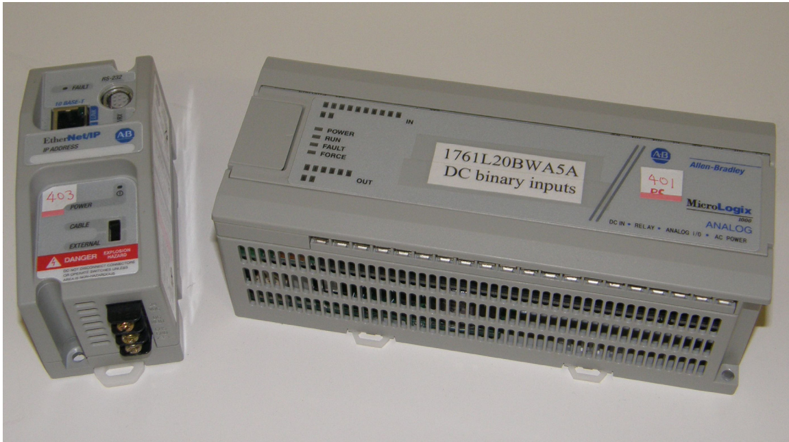
Figure 5-8. The Allen-Bradley MicroLogix 1000 PLC (on the right). This has analog and binary I/O ports. Its communications are handled by the 1761-NET-ENI unit shown on the left.
