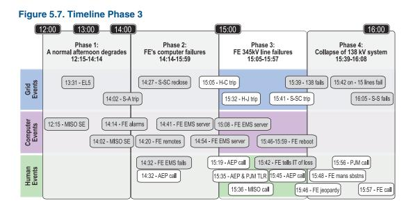
contacted a tree three times between 14:27:15 EDT and 15:41:33 EDT, opening and reclosing each time before finally locking out while loaded at 93% of its emergency rating at 15:41:35 EDT. Each of these three lines tripped not because of excessive sag due to overloading or high conductor temperature, but because it hit an overgrown, untrimmed tree.<sup>22</sup>
