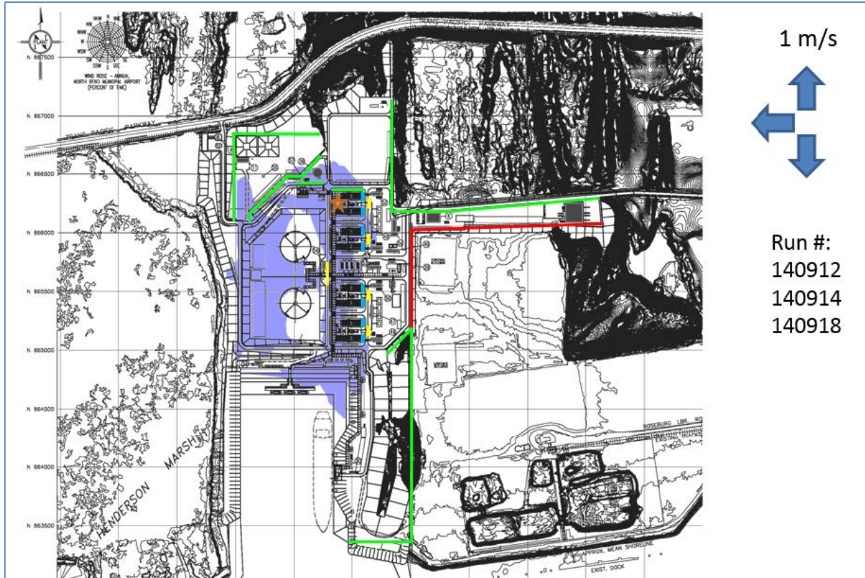
Figure 4.13-5. LNG Spill (i.e., Liquid Release Scenario) from a Guillotine Rupture of the Ship Loading Header into the Liquefaction Trench System (1 m/s)
