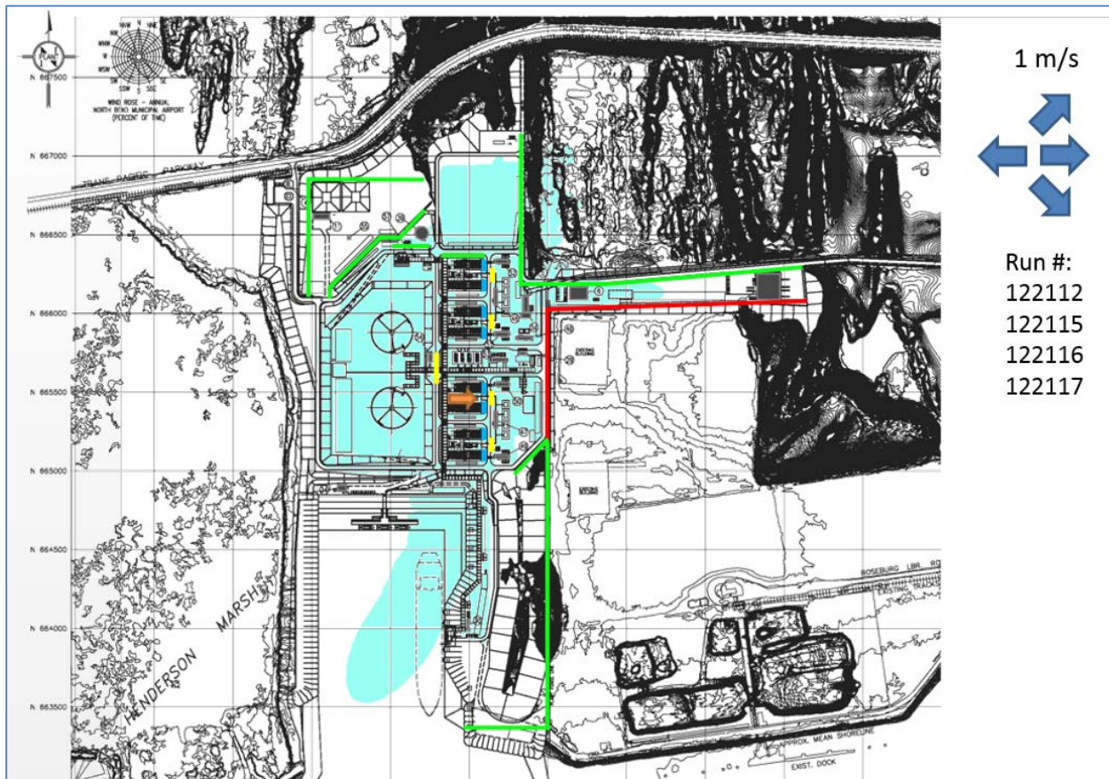
Figure 4.13-10. MR Release from Rupture of the Interstage Refrigerant Pump Discharge Piping (1 m/s)
