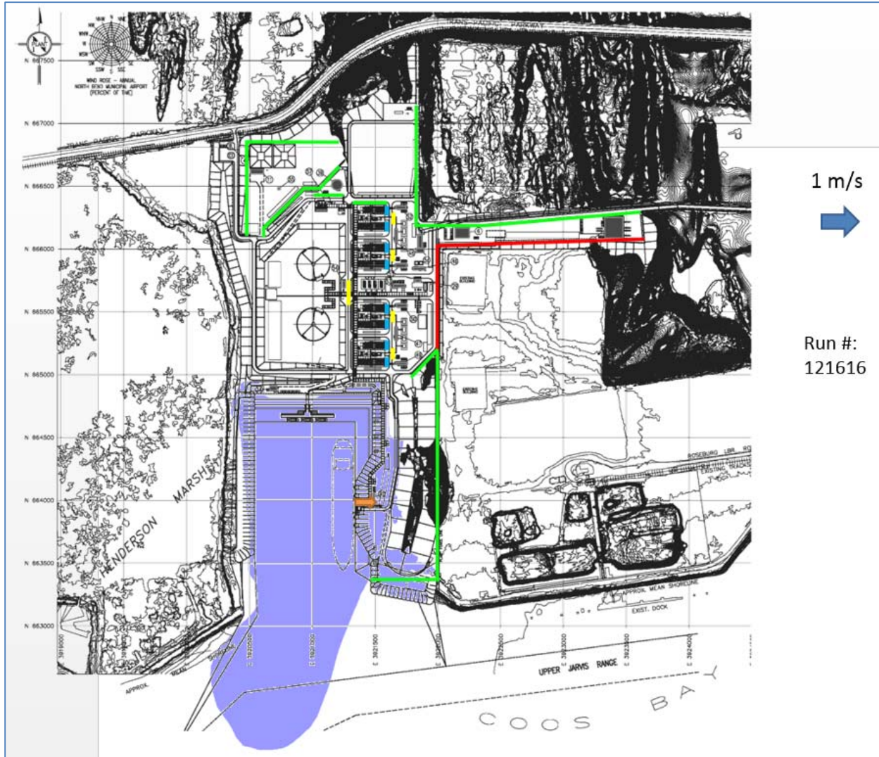
Figure 4.13-7. LNG Jetting and Flashing Scenario from a Rupture of the Ship Loading Header at the Marine Area (1 m/s)
