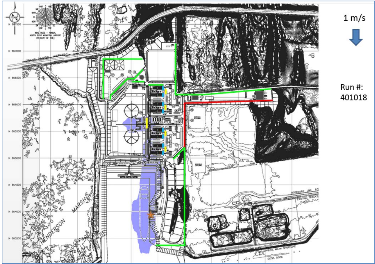
Figure 4.13-4. LNG Spill (i.e., Liquid Release Scenario) from a Guillotine Rupture of the Ship Loading Header into the Marine Berth Trench System (1 m/s)
