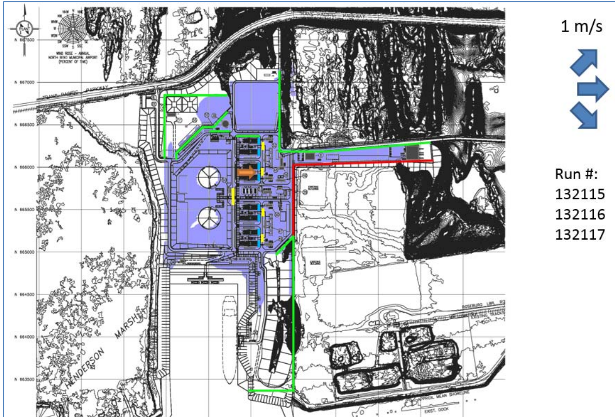
Figure 4.13-9. LNG Jetting and Flashing Scenario from a Rupture of the LNG Rundown Line at the Liquefaction Area (1 m/s)
