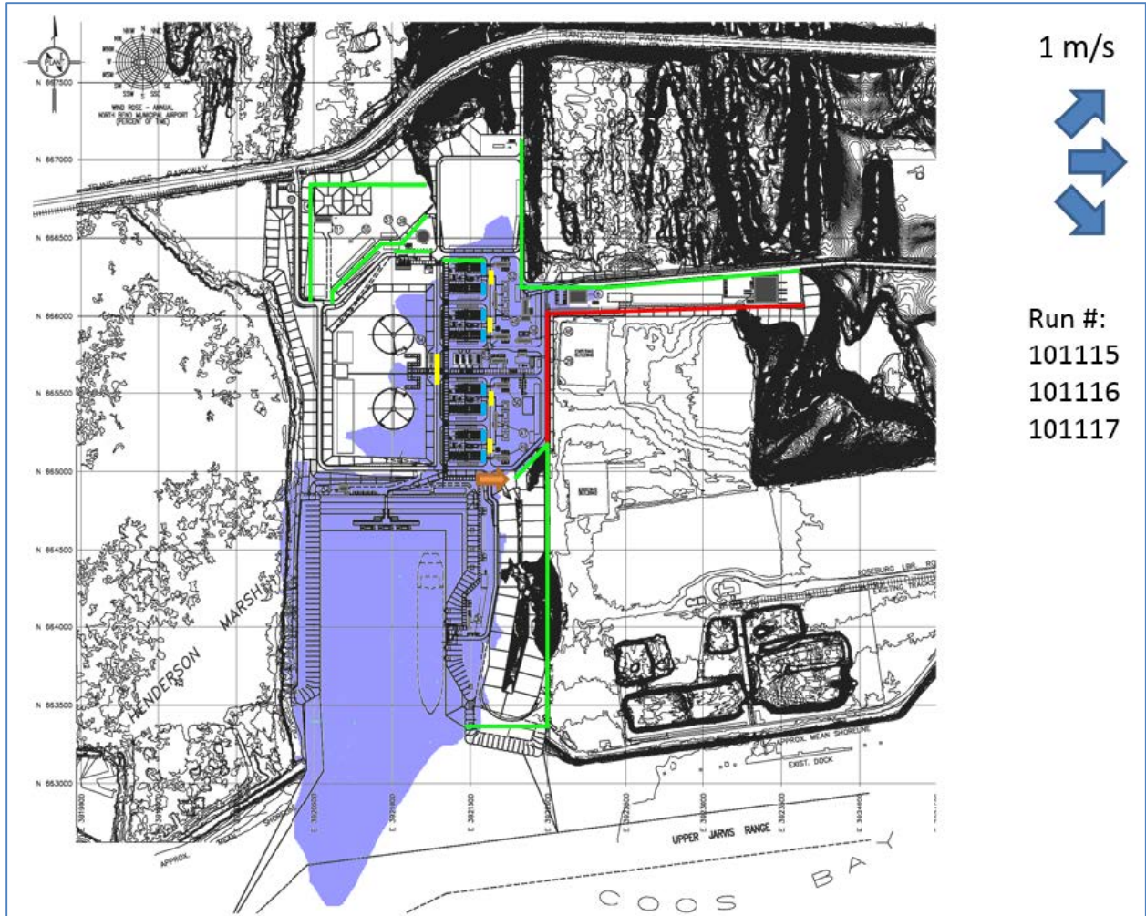
Figure 4.13-8. LNG Jetting and Flashing from a Rupture of the Ship Loading Header between the LNG Storage Tank Area and the Marine Area (1 m/s)
