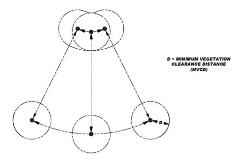
NERC indicates that conductor movements must be taken into account under FAC-003-2, and that the transmission owner is required to show that its approach to vegetation management under Requirement R3 will prevent encroachments under all expected line positions. Thus, a transmission owner must manage vegetation to ensure it does not encroach into the MVCD under multiple conditions.
