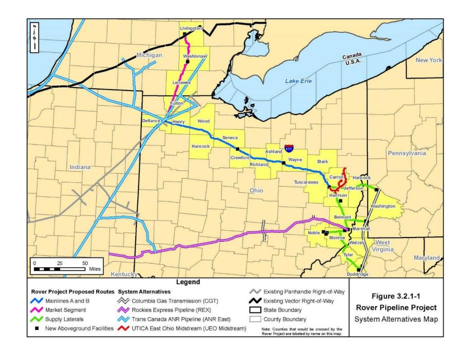
The UEO Midstream is in a similar geographic area, but has a different orientation than portions of the Clarington Lateral and the Supply Connector Lines A and B. More importantly; however, this pipeline system does not move processed transmission quality gas supplies; instead, it moves unprocessed gas to facilities to process the natural gas liquid components. For these reasons, we determined that it was not a viable system alternative.
