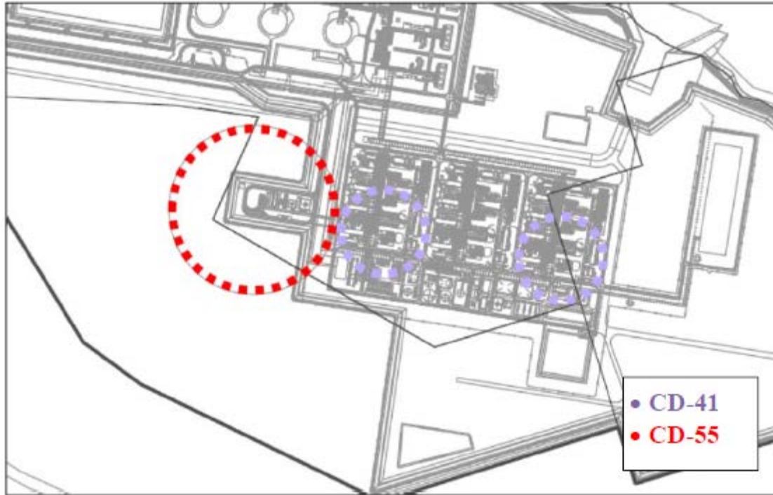
Figure 4.12.1-17 Maximum Extent of 1 psi from Condensate Overpressure Scenarios (property line shown in bold)
