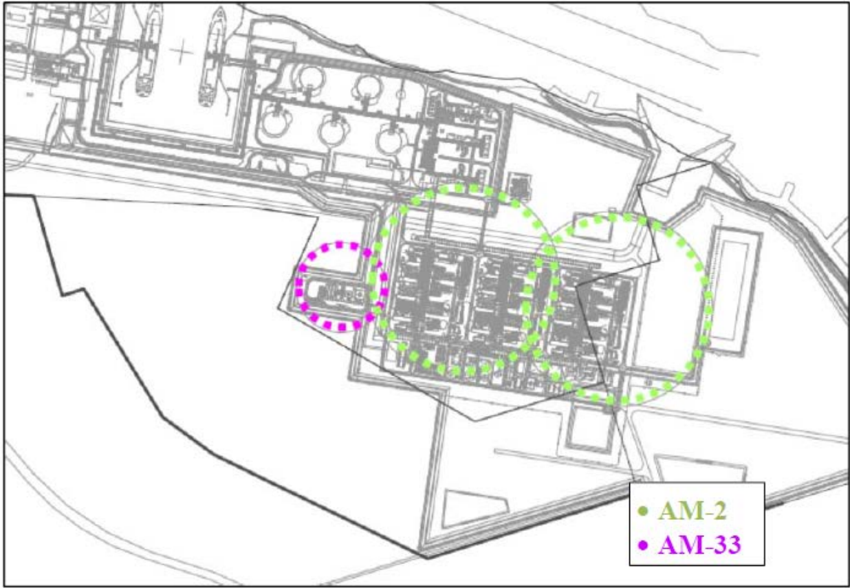
Figure 4.12.1-11 Maximum Distances to AEGL-1 for Ammonia Design Spills (property line shown in bold)
