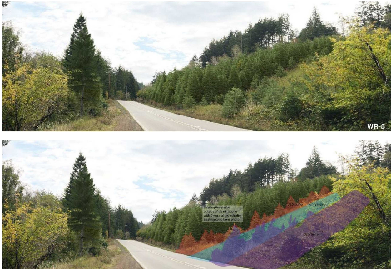
Figure K-12b. KOP-P10. Coos Bay Wagon Road (Near MP 24). Simulated site conditions five years after initial disturbance, repair and replanting (WR-5 above), and overlay of the proposed pipeline to illustrate location, showing the permanent 30-foot clear zone and the remainder of the initially cleared area.
