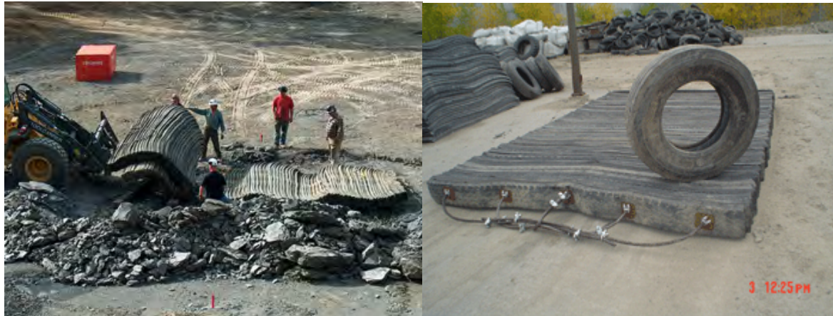
Photo 1 Typical Blast Mats Made from Used Tires
