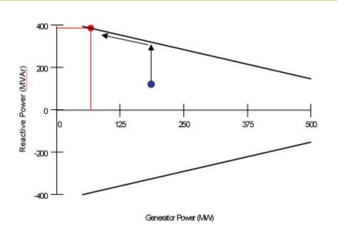
Figure 1. Generator A D-Curve and Operating Points, Case 1 and 2
