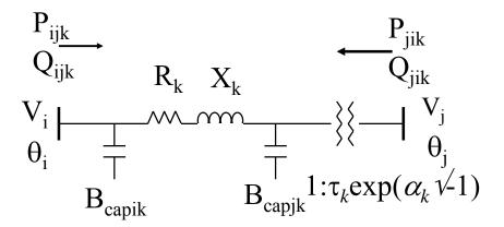
Shunt conductance in the model is omitted for clarity and since it is usually negligible. The basic equation for defining the real power flow along line k from bus i = I(k) towards bus j = J(k) is:
