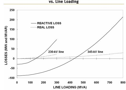
Figure 3: Transmission Line Real and Reactive Power Losses vs. Line Loading
