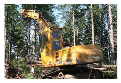
Yoader mobile shovel yarder configuration. Can utilize standing or live skyline setup for drifting carriages [motorized, Christy, buttrigging].
