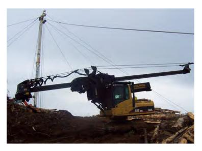
2) Tracked crawler-chipper. Unique machine comes in several horse-power and grinding capability configurations. The machine can crawl and grind on a range of slopes to process unmerchantable material at site of origin versus additional equipment that requires multiple-handling tasks of collection, skidding, and processing.
