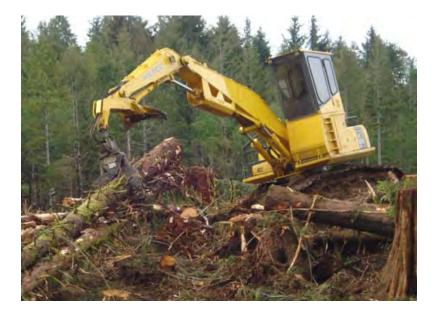
Dangle-head processor. Slope limited to +/-30%. Primarily delimbing, log manufacturing, and piling logs by species sort for efficient volume skidding. Production option.
