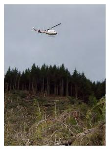
Dual engine and rotor helicopter configured for harvesting all sizes of timber.
