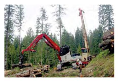
3) Yoader [aerial or ground-based]. Preferred base equipment is hydraulic heel boom log loader equipped with at least two winches. Mobile, extremely versatile, multi-tasking equipment: cable yard, log loading, shovel logging, tree pulling, slash piling. Needs minimal area for operation. Suited for cable yarding smaller timber, but can yard short length large diameter logs.
