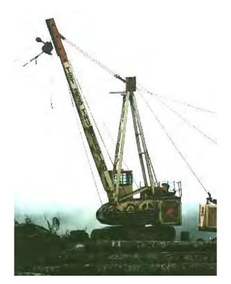
Rubber-tired self-propelled side-mounted cable yarder operating on narrow road width. Versatile configurations and mobile if safe access to tight rough terrain areas that can be yarder harvested.
