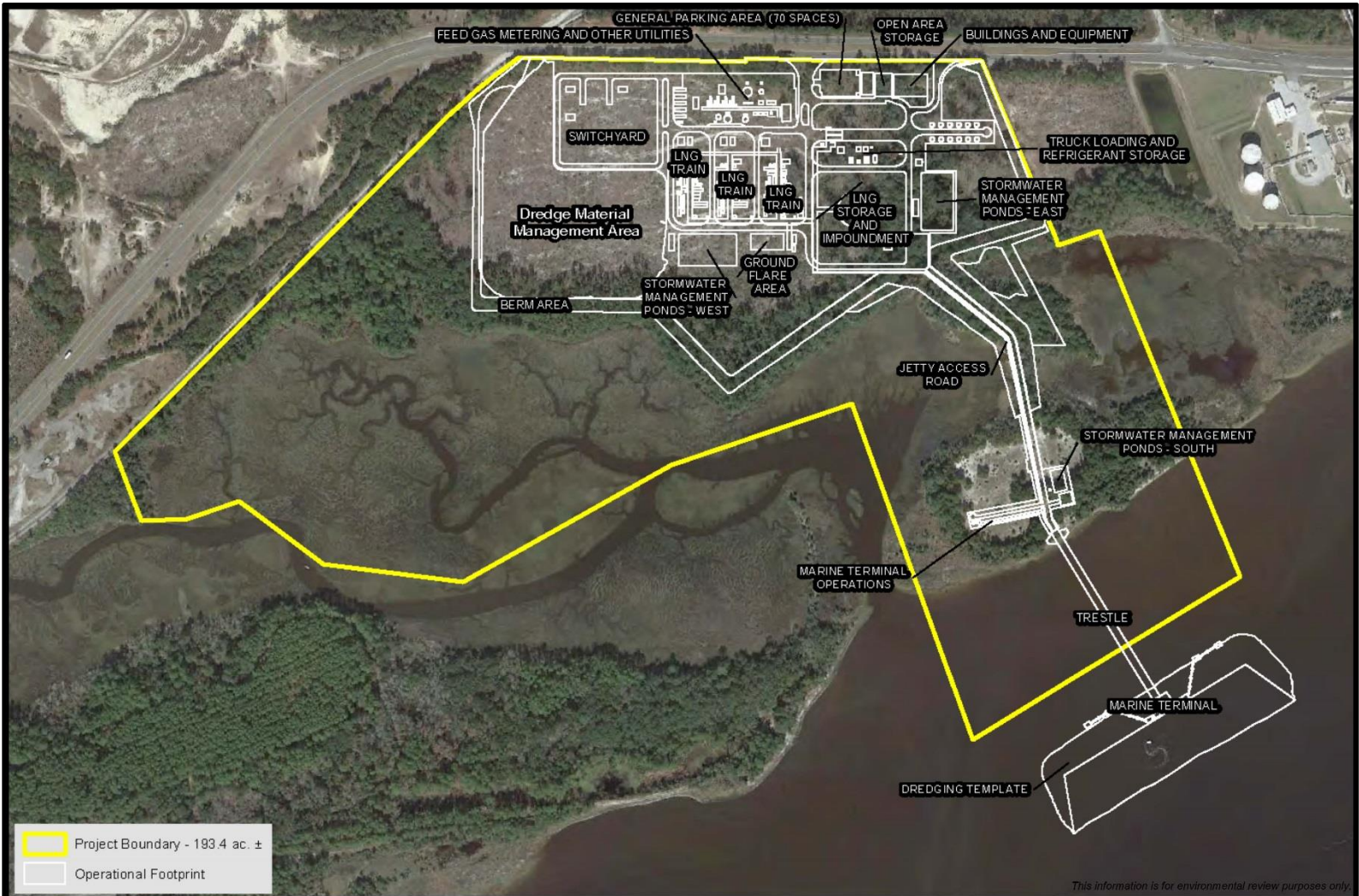
Figure 2.1.1-2 LNG Terminal Site Plan Jacksonville Project Duval County, Florida
