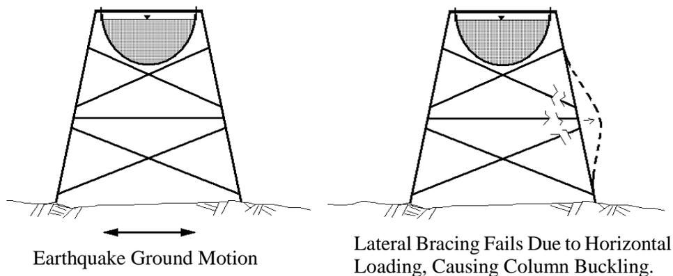
Fig. 16. Example of earthquake impact on the structural support for a flume.
