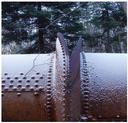
Fig. 6. Failed bellows expansion joint.
