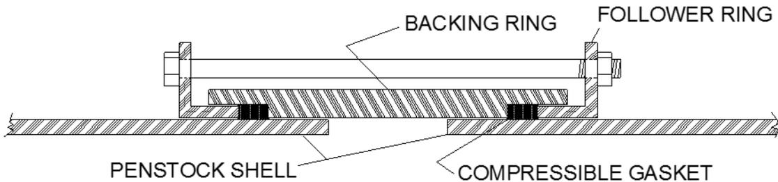
Fig. 5. Typical joint detail.
