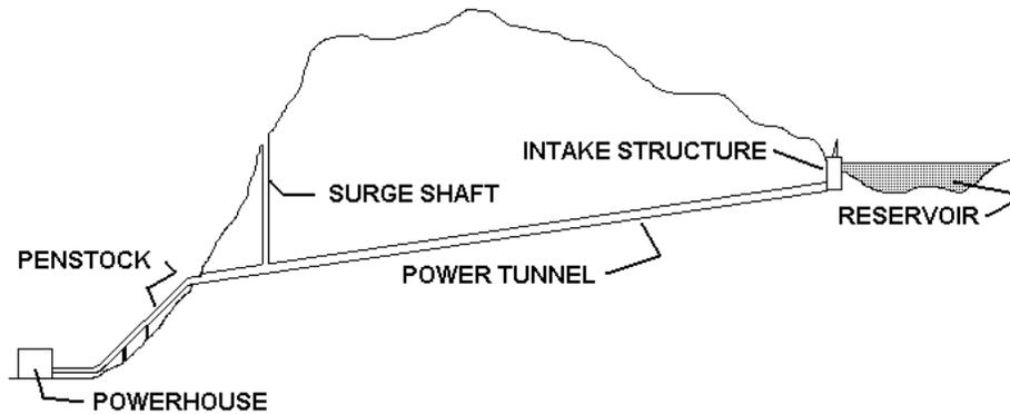
Fig. 17. Typical tunnel diagram.
