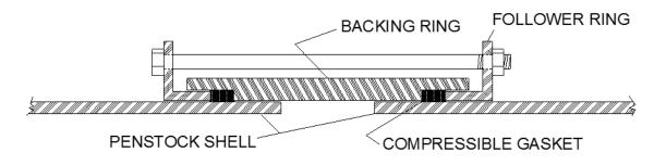
Fig. 5. Typical joint detail.
