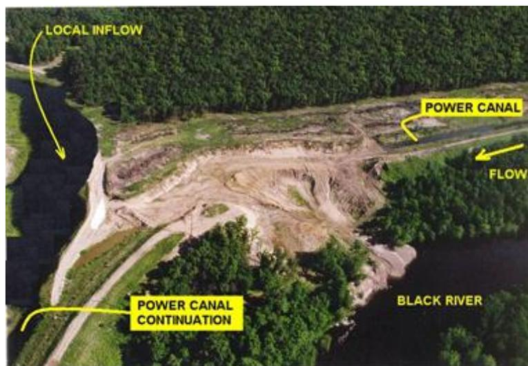
Fig. 9. Hatfield power canal failure.
