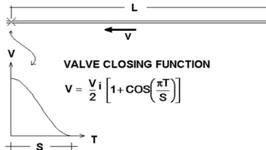
Fig. 3. Valve closing diagram.
