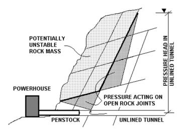
Fig. 19. Diagram of rock wedge at Schoellkopf.
