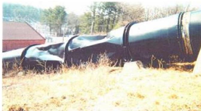
Fig. 4. Buckled steel penstock.
