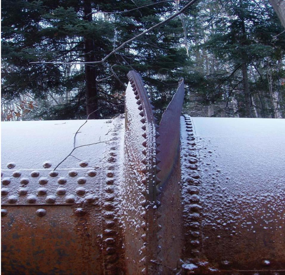
Fig. 6. Failed bellows expansion joint.
