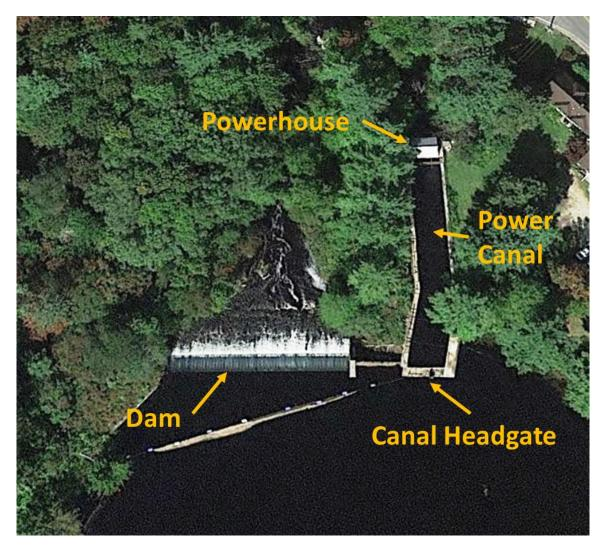
Fig. 7. Typical power canal layout (Powder Mill Pond, Google Earth).
