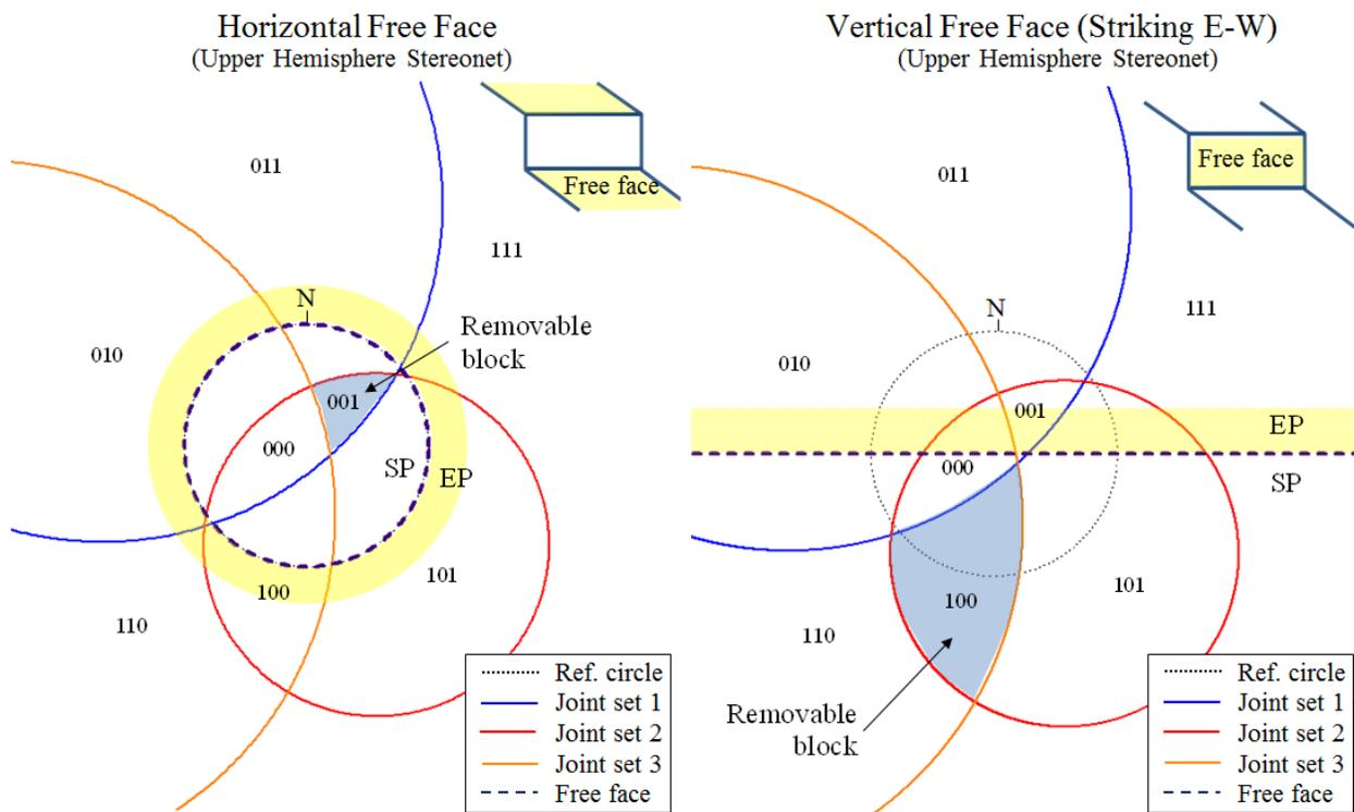
Figure 11A-14 - Upper hemisphere, equal angle stereonet showing JP codes and removable blocks for horizontal free face (left) and vertical free face striking East-West (right) (George, 2015).
