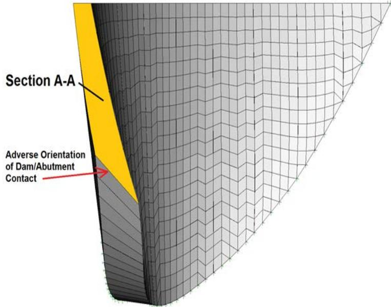
Local sliding will occur, which will deny the arch necessary support. The stress plot below shows the flow of stress around this area. Note the stress' tendency to dive below the area of adverse orientation.
