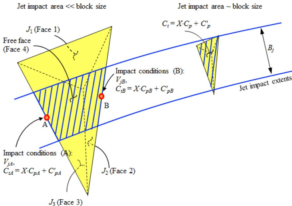
Figure 11A-17 - Loading scenarios for removable blocks subject to block size relative to jet impact area.
