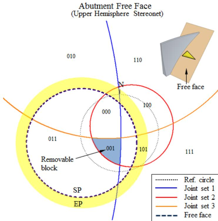
Figure 11A-20 - Upper hemisphere equal angle stereonet showing JP codes and removable block for the dam abutment slope.
