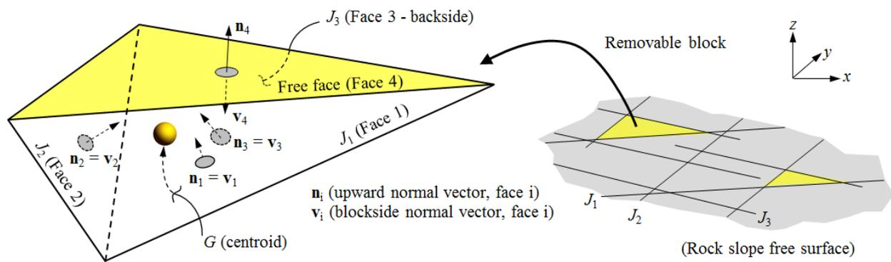
Figure 11A-16 - Removable block schematic (George, 2015).
