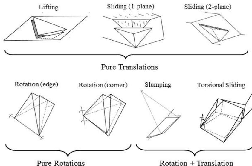
Figure 11A-15 - Kinematic block failure modes (Goodman, 1995).
