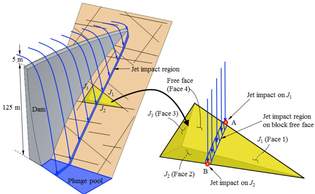
Figure 11A-19 – Schematic of overtopping jet onto removable abutment block.
