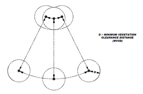
NERC indicated that conductor movements must be taken into account under FAC-003-2, and that the transmission owner is required to show that its approach to vegetation management under Requirement R3 will prevent encroachments under all expected line positions. Thus, a transmission owner must manage vegetation to ensure it does not encroach into the MVCD under multiple conditions.
