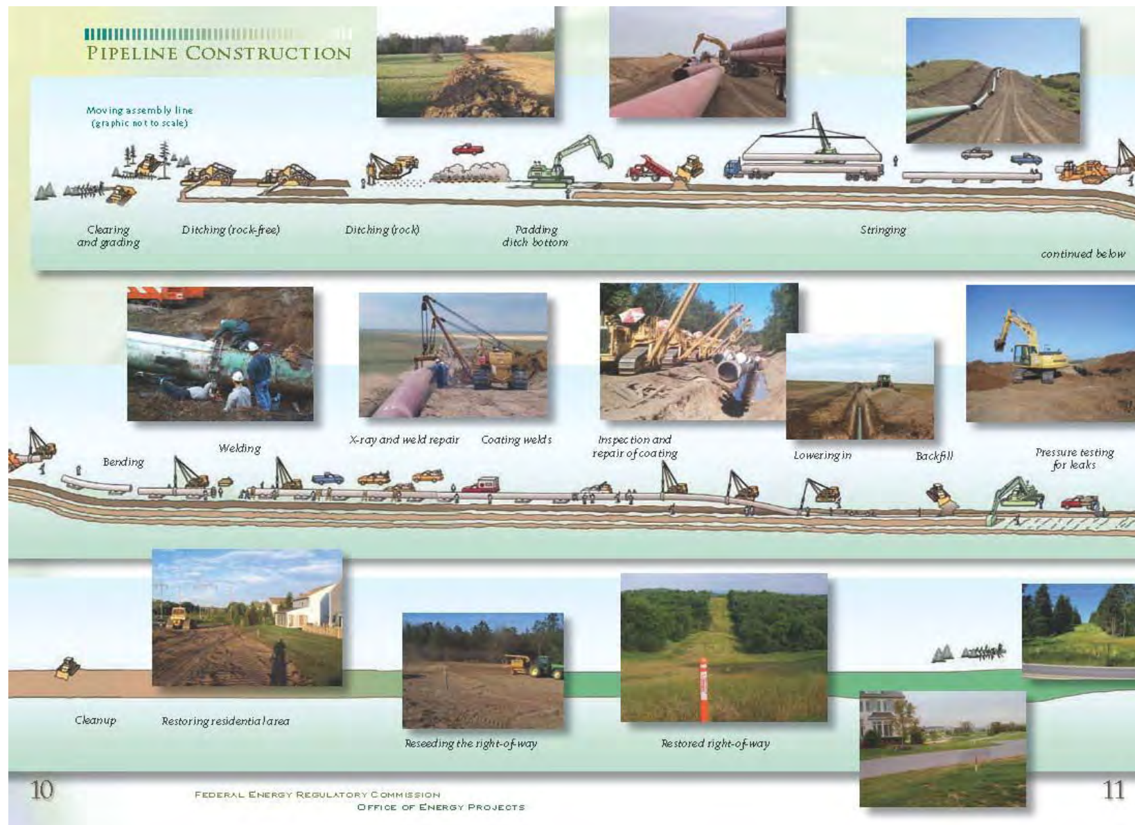
Figure 2: General Pipeline Construction Sequence
