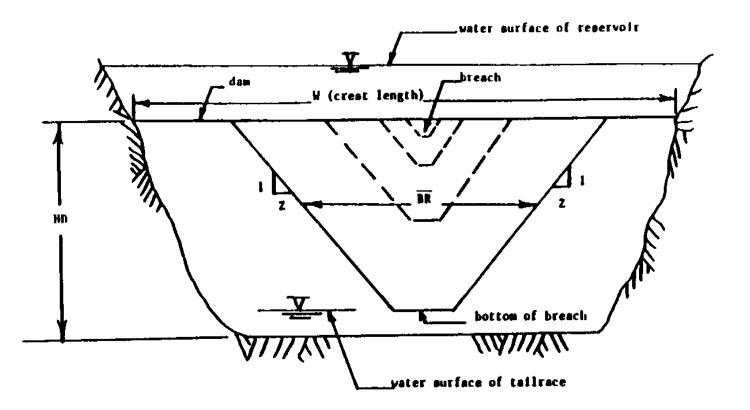
FIGURE 1. DEPINITION SKETCH OF BREACH PARAMETERS
