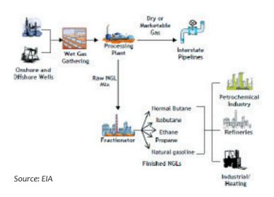
Once a well is completed and production starts, the natural gas moves into gathering pipelines, typically small-diameter lines that move the gas from the wellhead to either a processing plant or a larger pipeline.
