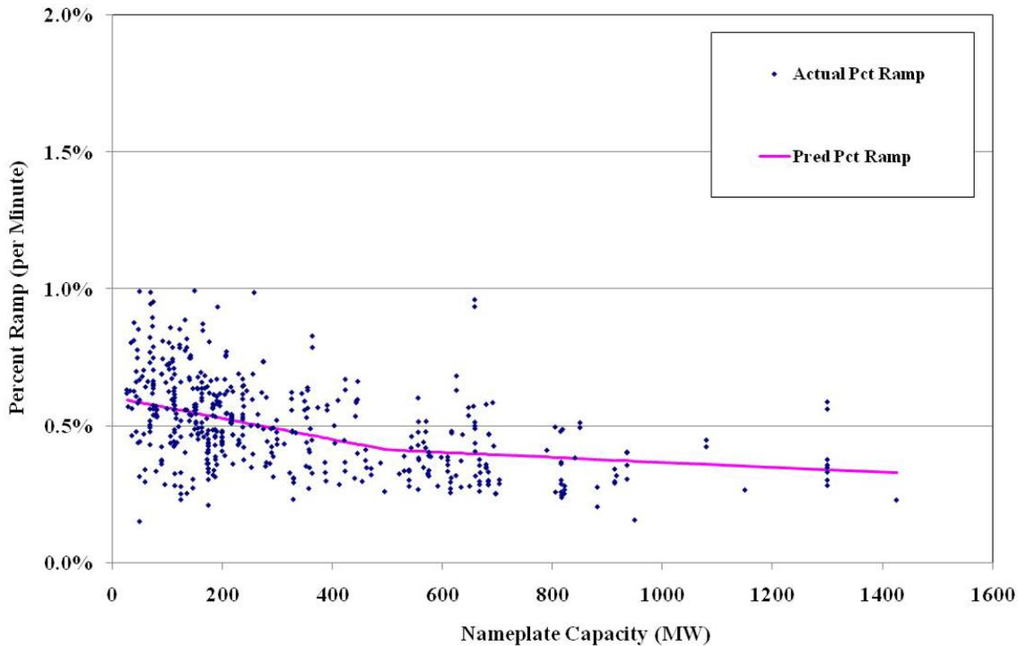
**Figure 1: Percentage Up Ramp as a Function of Nameplate Capacity, Steam Units, PJM, 2010**
