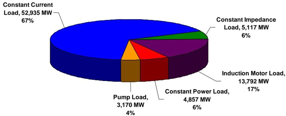
**Figure 2-2. Western Interconnection Load Composition - 2012 Minimum System Load**
