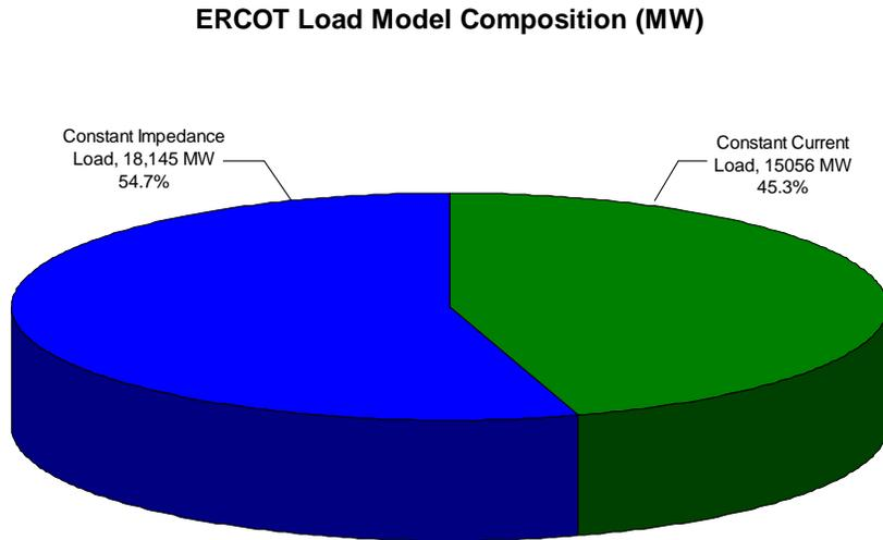
**Figure 3-2. Texas Interconnection Load Composition - 2012 Light System Load**
