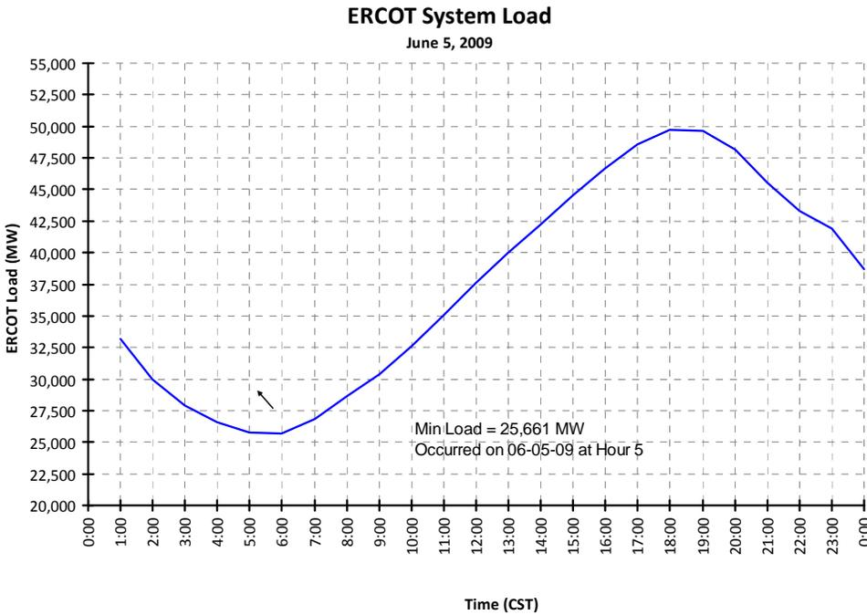
**Figure 3-1. Texas Interconnection System Load – June 5, 2009**
