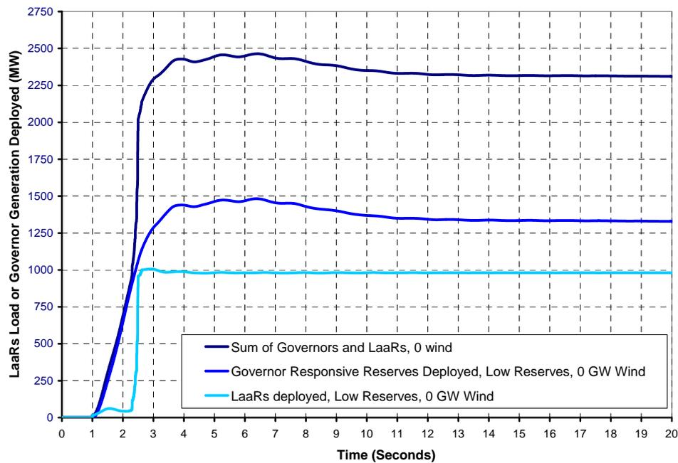
**Figure 3-5. The Power Delivered (and Load Removed) by Primary Frequency Control Actions via Generator Governors and Load Acting as a Resource following the Sudden Loss of 2,450 MW of Generation – Low Reserves and 0 GW of Wind**
