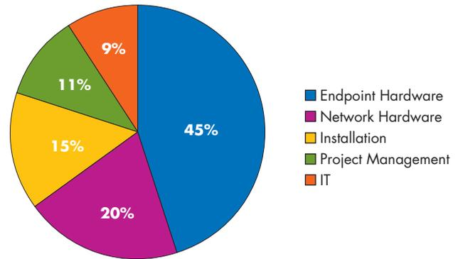
Figure 2: AMI System Cost<sup>1</sup>
