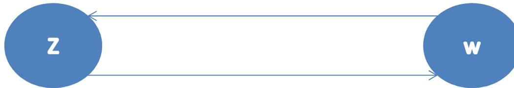
A 1 MW increase in the TTC of the connection in both directions yields the same reliability effect as building  $X_z$  of UCAP in zone z or  $X_w$  of UCAP in zone w where
