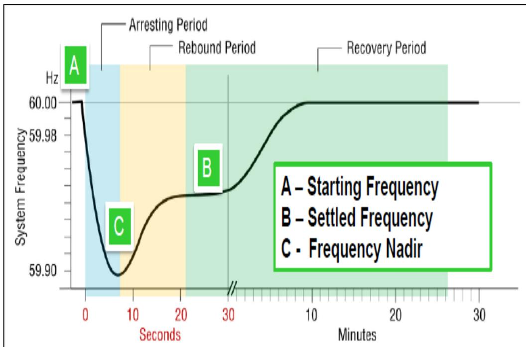
Figure 2: Typical frequency response following a generator trip.
